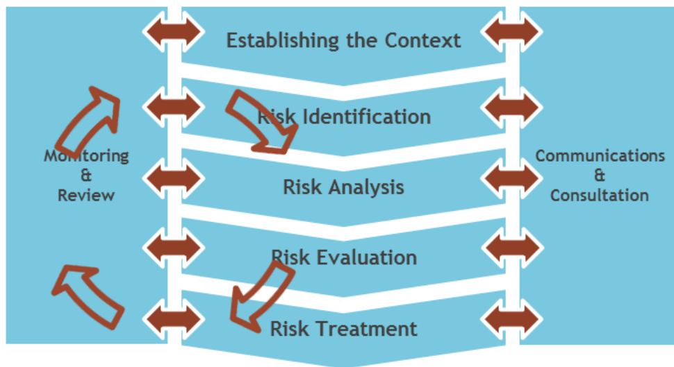
Figure: Monitoring & Risk Assessment Cycle as part of the ISO 31000 risk management process
